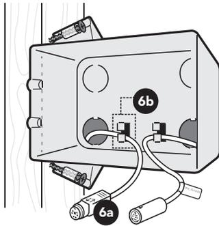
**IMPORTANT NOTE:** Be careful not to strain, staple, pinch or otherwise damage the cables. Route cables as required to permit replacement. Do not route cables inside conduit together with power lines or close to hot water or steam piping.
