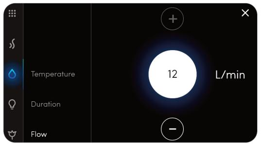
Tap Flow to adjust the volume of the shower. Use the + and – buttons to adjust the volume.
