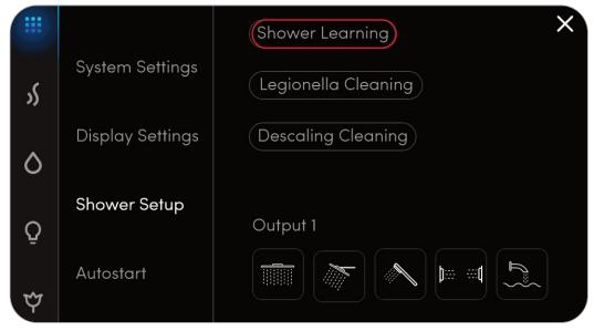
Navigate to Shower Setup in features menu and press Shower Learning. The hot and cold supply must be on and the shower fixtures MUST be connected. The control will display a message that says the shower learning is in progress. While the learning is taking place the outputs will open and close to learn the flow characteristics of each fixture.
