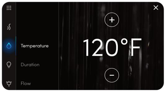
Tap Temperature to adjust the temperature of the shower. Use the + and – buttons to adjust the temperature.
