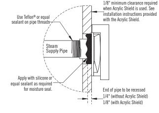
Consult with supplier of acrylic, fiberglass and other non-heat resistant enclosures for recommended steamhead location. Use Acrylic Shield PN 103938/ 103938SQ. See instructions provided with steam shield. (An acrylic shield is not available for the iSteam steamhead.)
