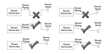
for condensate to drain, may cause condensate to block the flow of steam. Blocking the steam flow may cause steam pressure to discharge boiling water through the steamhead, resulting in a scalding hazard. Blocking the flow of steam may cause steam to discharge through the safety valve, resulting in a scalding hazard.
