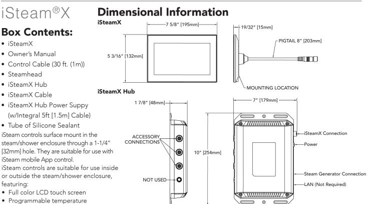
The iSteam controls are designed to be installed inside or outside the steam room but is primarily installed inside the steam room. If the control is installed inside the steam room the control must be located:
