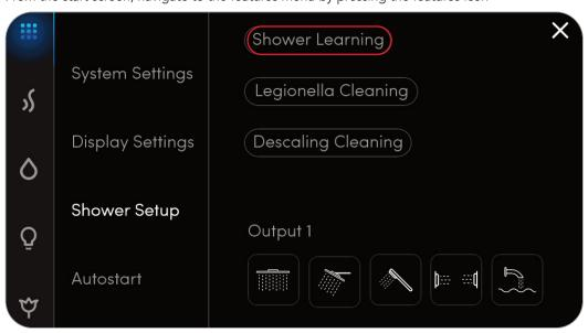
Navigate to Shower Setup in features menu and press Shower Learning. The hot and cold supply must be on and the shower fixtures MUST be connected. The control will display a message that says the shower learning is in progress. While the learning is taking place the outputs will open and close to learn the flow characteristics of each fixture.
