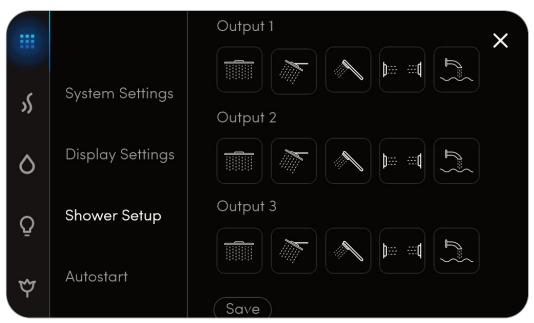
Once the shower leaning has been completed, each output can be assigned a fixture icon (note each may only be used once) Select the icon the corresponds to the output, once the selections are made press SAVE. Note: If an output is not plumbed you will not be able to make a selection for it
