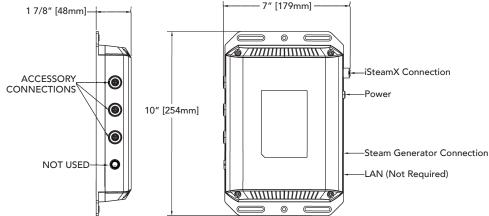
The iSteam controls are designed to be installed inside or outside the steam room but is primarily installed inside the steam room. If the control is installed inside the steam room the control must be located:
