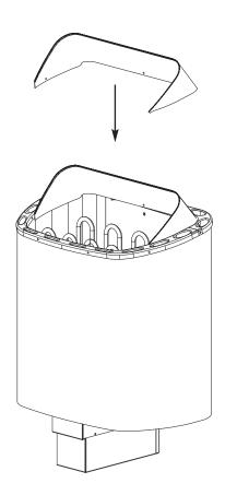
**8.** Remove the heat shield from the heater and secure it in place using the 3 screws provided.
