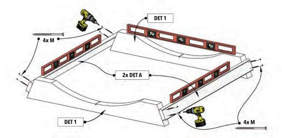
CAUTION Ensure the base is level, and the boards are spaced evenly front to back and side to side before continuing to prevent issues later in the build.
