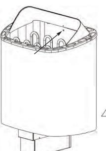
To prevent a shock and burn hazard, the heater must be screwed to the bracket as shown.
