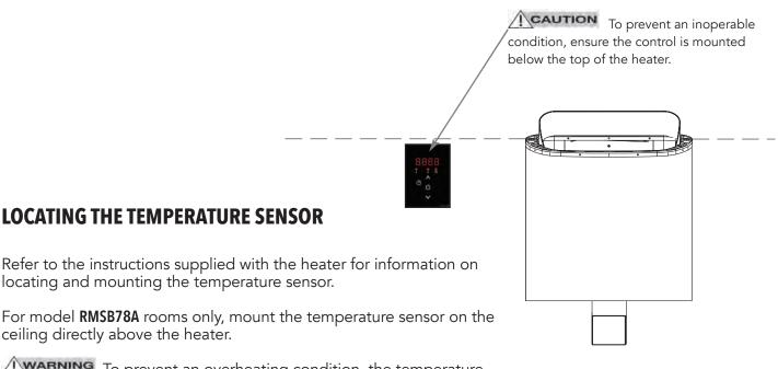
**WARNING** To prevent an overheating condition, the temperature sensor must be located per these instructions.
