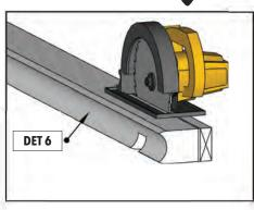
If needed, trim the flat edge of the board to create the desired width.
