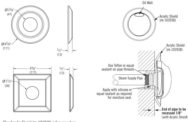
The Acrylic Shield (PN 103938) is for use when acrylic or other non-heat resistant materials are used for the steamroom enclosure.
