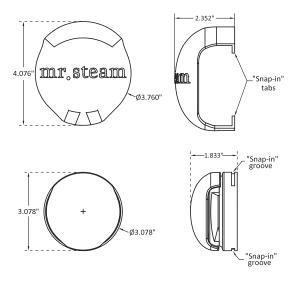
FOR ILLUSTRATIVE PURPOSES ONLY. IMPORTANT NOTE: FOR SAFE AND TROUBLE FREE INSTALLATION Before installation, visit mrsteam.com to download the Installation, Operation and Maintenance Manual or refer to the manual provided with the unit.
